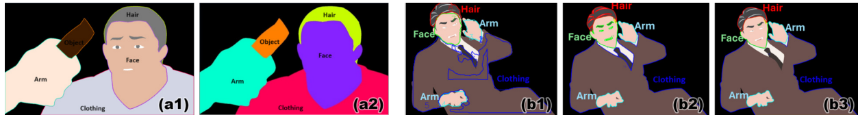
Figure 7: (a1 and a2) Annotated contour and layer masks, respectively, using our annotation tool. (b1) YOLOv5 object detection and instance segmentation results. (b2) Flat based segmentation contours. (b3) Overlap identification and flat contour merging.
